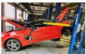
Another sad story: An owner of a new C8 Vette took his car to the dealer and supposedly the techs improperly lifted his car, causing it to fall off the lift and land hard on the shop floor. The impact caused body damage to the car and broke out the windows.
